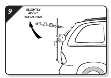
Reposition the cycle support arm so it is positioned slightly above horizontal.
